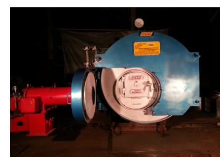
3 TPH Solid Boiler
